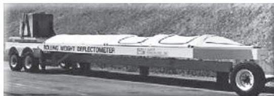
写真-13 Rolling Weight Deflectometer<sup>14)</sup>
