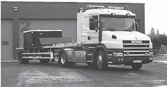
写真-16 High Speed Deflectograph
